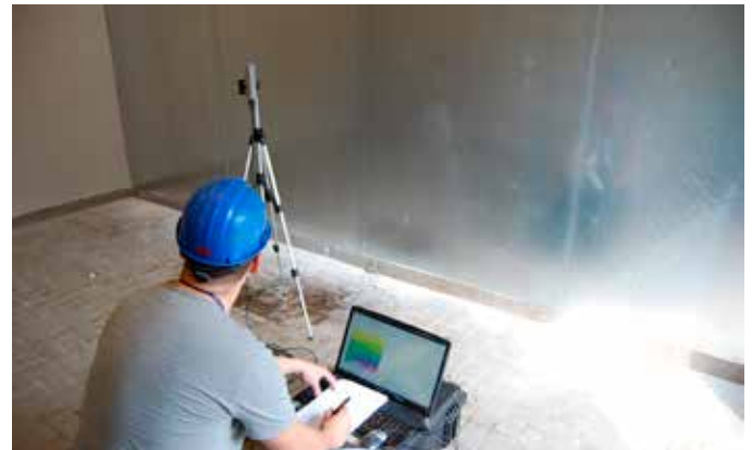
Magnetic field-strength measuring after shielding
